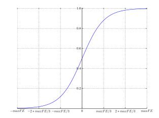
Fig. 1. Sigmoid Function Used in Adaptive Collision Scheme
