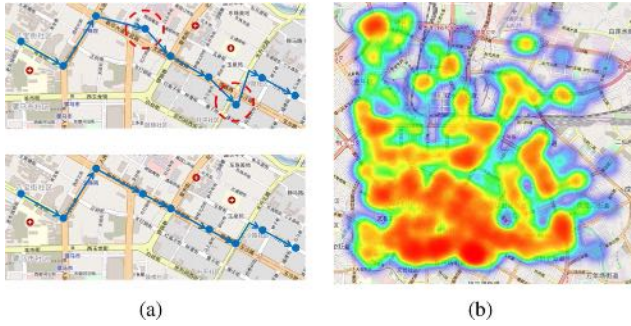
Fig. 2. (a) Illustration of map matching. Upper: Original trajectory points; Lower: Map-matched trajectory points. (b) Heatmap of trajectory points in Chengdu (The deeper color indicates a more dense distribution of trajectories).
